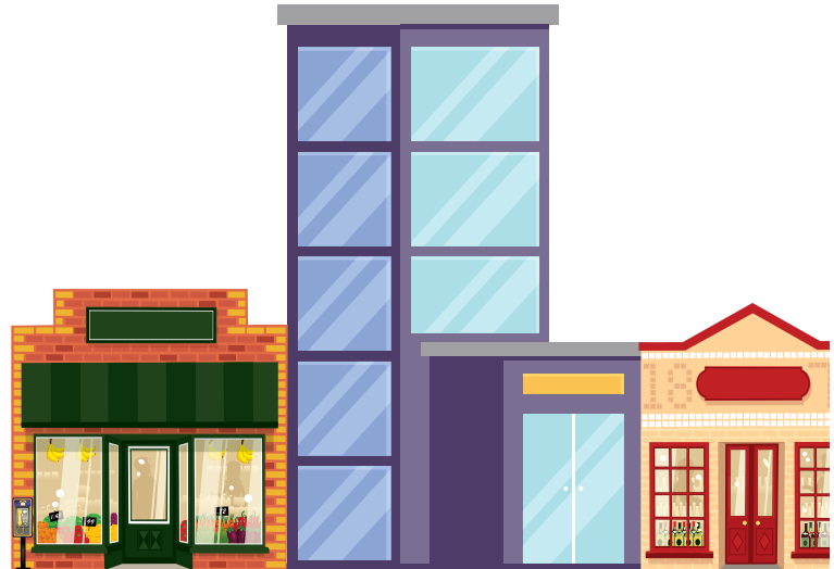
Figure 3.4. Compatible infill should respect the scale and height of surrounding historic buildings. In this illustration, the new building in the center is several stories taller than the adjacent buildings, impacting the scale of the streetscape.
